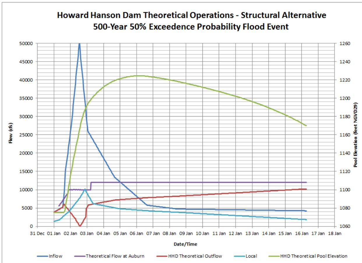
Figure 4-3: HHD Operations Model Results for 0.2% AEP Median Flood Event, Structural Alternative
